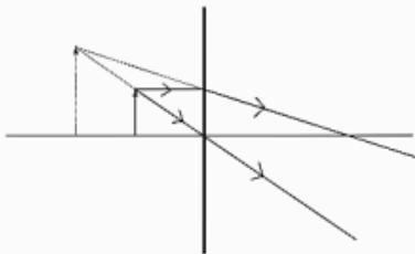
The above figure shows the formation of an image by a lens shown by a thick line. [2 Marks]
