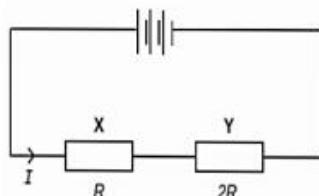
The above figure shows two resistors X and Y connected in series to a battery. The power dissipated for this combination is  $P_1$ . When these resistors
