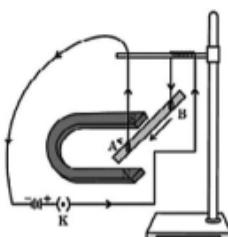
A student was asked to perform an experiment to study the force on a current carrying conductor in a magnetic field. He took a small aluminum rod AB, a strong horse shoe magnet, some connecting wires, a battery and a switch and connected them as shown. He observed that on passing current, the rod gets displaced. On reversing the direction of current, the direction of displacement also gets reversed. On the basis of your understanding of this phenomenon, answer the following questions:
