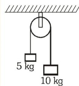
6. Two blocks of masses 5 kg and 10 kg are connected to a pulley as shown. What will be their acceleration if the pulley is set free? ( $g = 10 \text{ ms}^{-2}$ )
