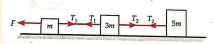
14. As shown in fig, three masses  $m$ ,  $3m$  and  $5m$  connected together lie on a frictionless horizontal surface and pulled to the left by a force  $F$ . The tension  $T_1$  in the first string is 24 N. Find (i) acceleration of the system (ii) tension in the second string (iii) force  $F$ .
