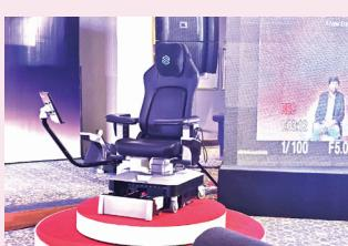
It is a fully integrated, ergonomic, and compact telesurgery console designed to allow expert surgeons to perform complex surgeries remotely. The system utilises magnetic sensor-based controls and lightweight 3D glasses, enabling high-precision operations in real time. Developed by a team led by Dr Sudhir Srivastava, Founder and Chairman of SS Innovations International, the console demonstrates India's growing capability in advanced medical technology innovation.
