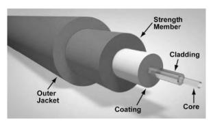
In optical fibre cable light pulses bounce back and transmit from one place to
