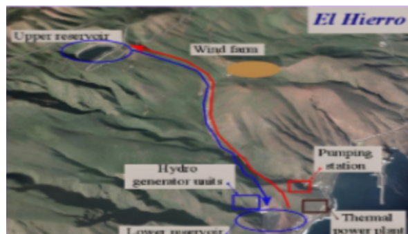
Fig. 4 Main elements of the hydro-wind power (Interconnection schematic Diagram)
