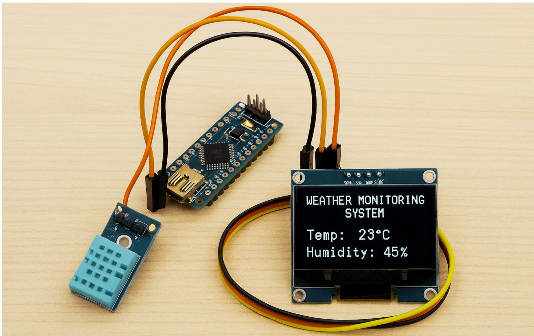
The weather monitoring system uses the DHT11 sensor to measure temperature and humidity from the surrounding environment. The sensor sends this data to the Arduino Nano, which processes the information. The Arduino then displays the real-time temperature and humidity readings on a small OLED screen, allowing users to easily monitor weather conditions. This project helps students learn about sensor integration, data acquisition, and display programming using microcontrollers.
