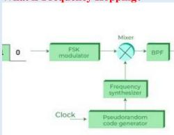
Frequency hopping is a technique that allows a signal to rapidly switch between different frequencies, making it difficult for an enemy to jam or intercept the signal. This technique is particularly useful for military applications, as it ensures secure communication even in hostile environments.
