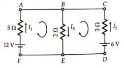
20. Find the potential difference across each cell and the rate of energy dissipation in R.
