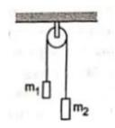
27. Consider the situation shown in figure. All the surfaces are frictionless and the string and the pulley are light. Find the magnitude of the acceleration of the two blocks.
